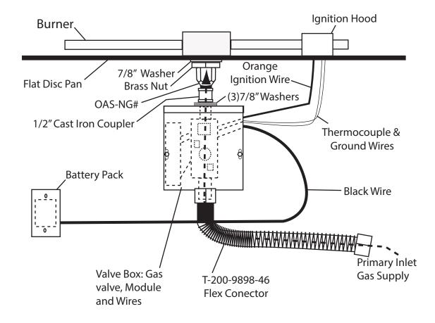
**Note**: Use joint compound or Teflon tape resistant to all gasses on all male NPT threads; not flared fittings. Ensure all connections are tight and check for gas leaks before and after assembly is complete.
