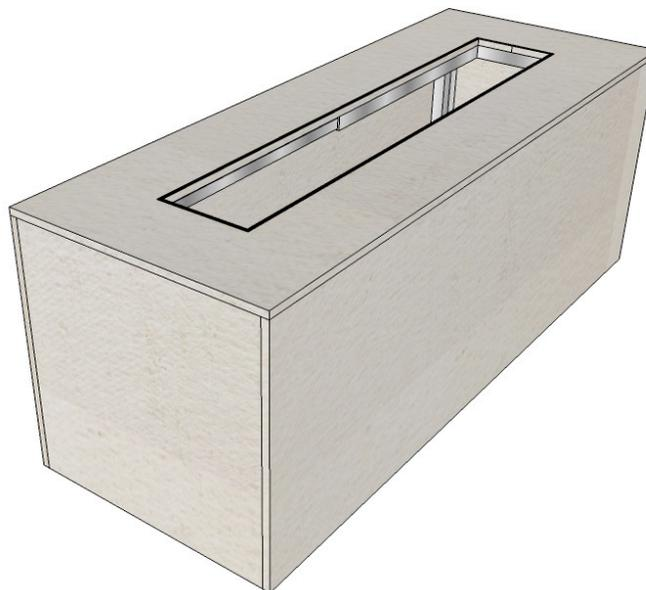
Use the 1¼", grey coated screws that are included in the kit to fasten the top panels to the outer perimeter framing and burner supports. It is best to pre-drill the holes through the board material and into the steel tubing using a 1/8" drill bit prior to installing the screws.
